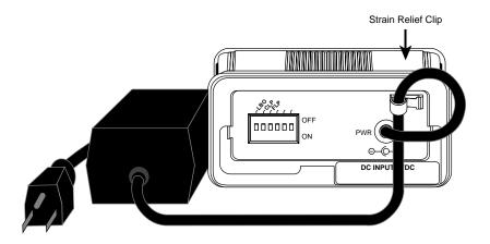
If an additional extension cord is used to connect the power module to the power source, the following guidelines must be followed.
